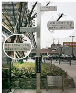
The Raising Water Level at the Past Typhoon Flood at JR Amagasaki Station
